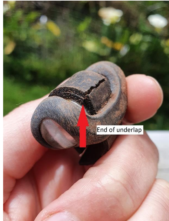
Fig. 3. A CEFAS TDR in a cast-mould mount showing where the neoprene rubber straps disintegrated. Credit: K. Simister.
